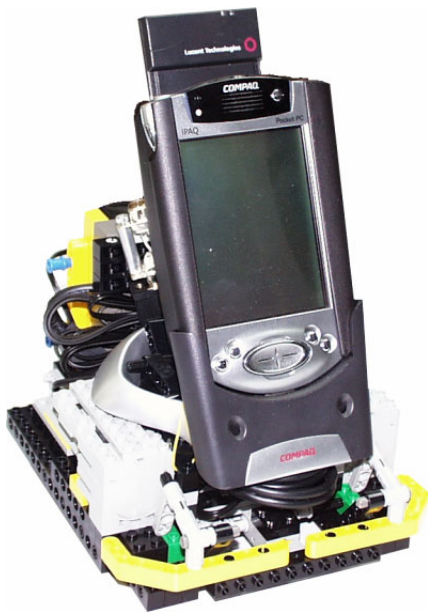
Figure 4: Robot with PDA for WLAN communication
